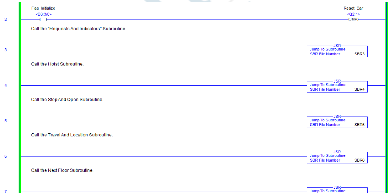
Figure 5. Ladder logic of Rung 3 to Rung 7
