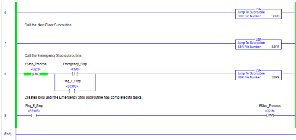
Figure 6. Ladder logic of Rung 8 and Rung 9
